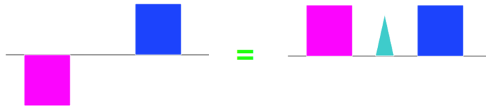
Figure 16.22 The gradient echo in a spin echo experiment: the effective gradient (need to label pulse with a 180°)
